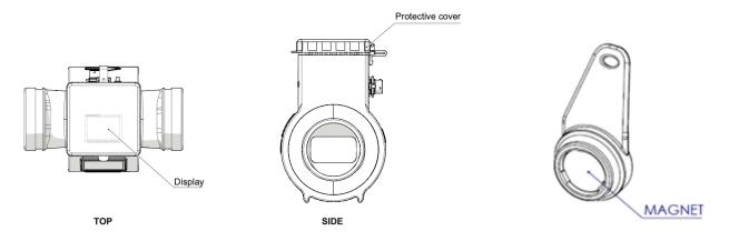
The MUT 7000 meter is equipped with a magnet for magnetic reed operation.
